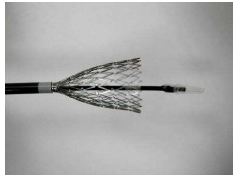
A self-expanding nickel titanium stent emerging from its delivery catheter. Devices like this are engineered to contract to less than 1 mm in diameter for delivery into a blood vessel and expand to full size when deployed (as in the picture).
