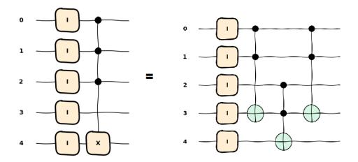
The first Toffoli gathers the information from wires 0 and 1 and stores it in the ancilla located at wire 3. The second Toffoli then uses the information on wire 2 and the ancilla to control wire 4, our target wire. Finally the third Toffoli uncomputes the ancilla, returning it to the  $|0\rangle$  state.
