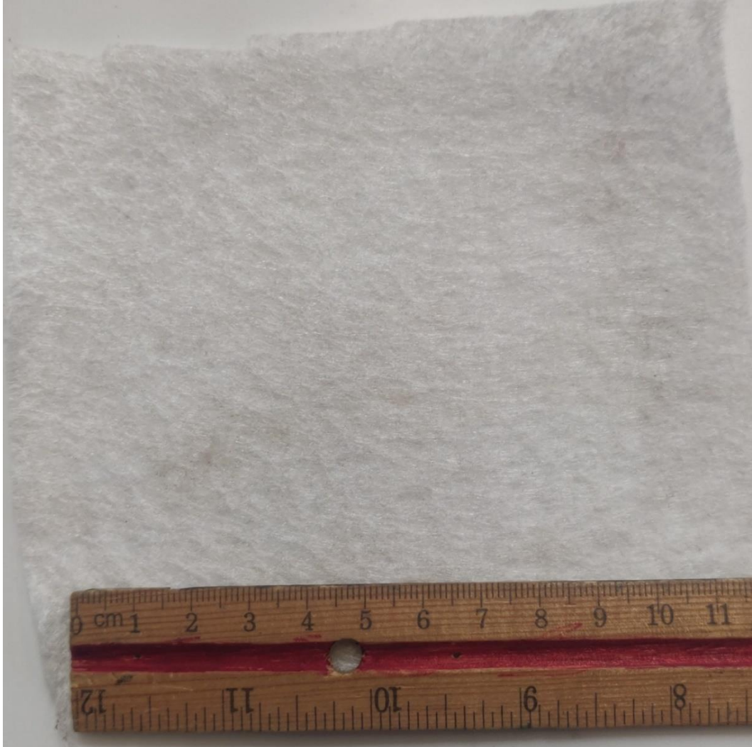
Figure S5.1 Needle punched non-woven geotextile with a characteristic opening size ( O_{90} ) of 100\ \mu\text{m} (\pm 30) .
