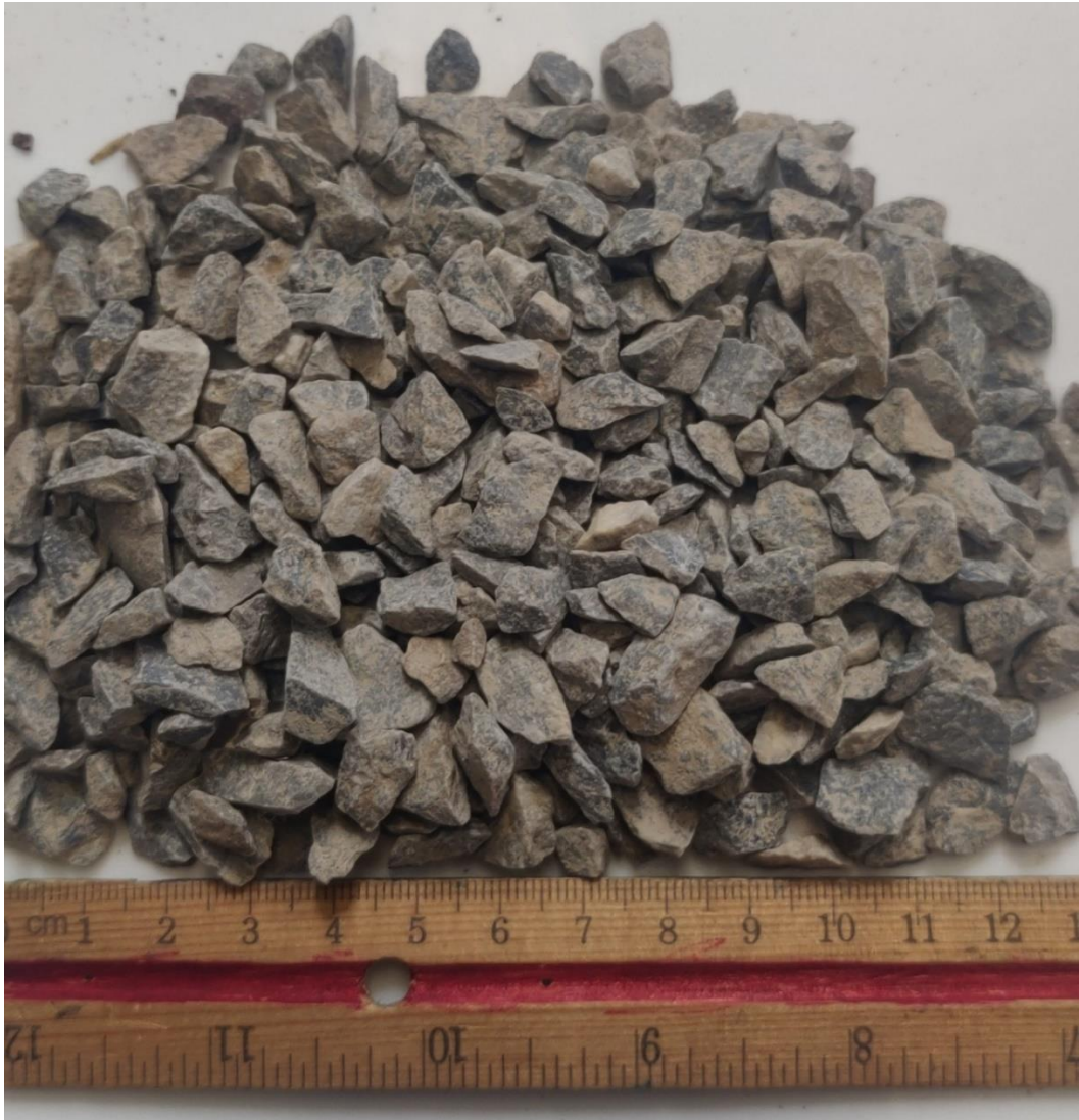
Figure S5.3 Chipped limestone with a gradation of 2-10 mm (D 15 -D 75 ).
