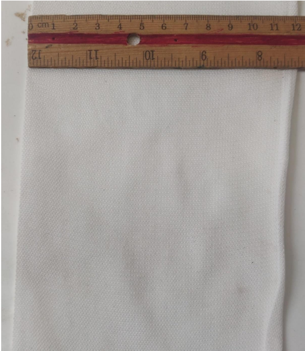
Figure S5.2 Knitted polyester filter sock with an O_{90} of 150 – 200 \mu\text{m} .
