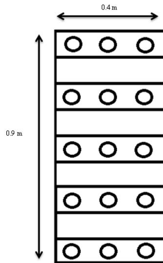
**Figure 3.3.** Calibration area and positions of collection containers
