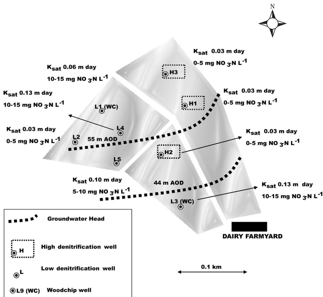
Fig. 1. Schematic of dairy farm site with location of woodchip (WC) wells, wells with high (H) and low (L) denitrification potential,  $NO_3^-$  ranges and  $K_{sat}$  for each well.
