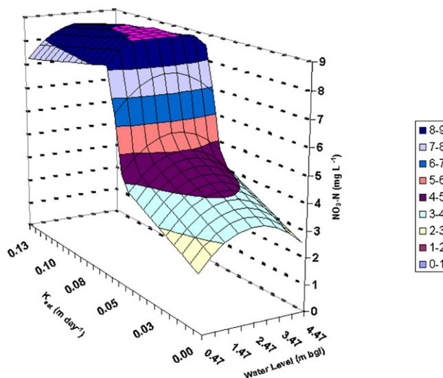
Fig. 4. Predicted NO<sub>3</sub>-N model using K<sub>sat</sub> and water level.
