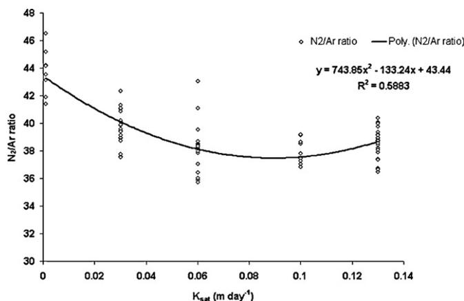
Fig. 5. Relationship between physical (K<sub>sat</sub>) and denitrification (N<sub>2</sub>/Ar ratio) parameters.
