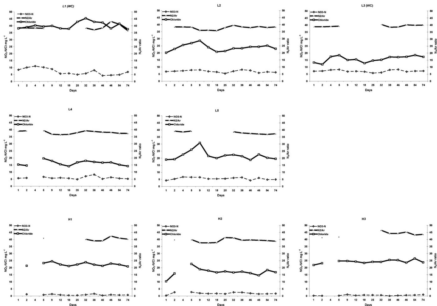
Fig. 2. Groundwater  $N_2/Ar$  ratios,  $NO_3-N$  ( $mg\ L^{-1}$ ) and  $Cl$  ( $mg\ L^{-1}$ ) concentrations for low (L1–5) and high (H1–H3) denitrification potential wells over time. WC here signifies presence of woodchip.
