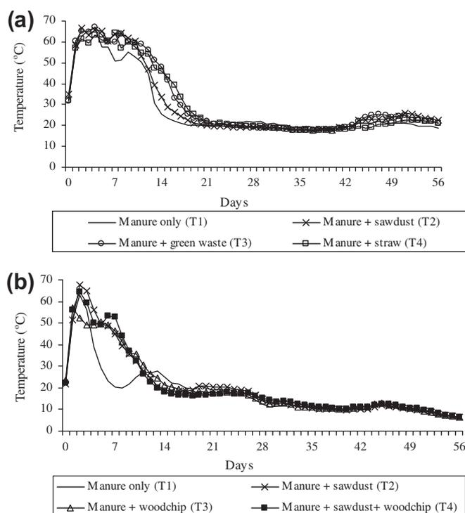
**Fig. 2.** Compost temperature for Trial 1 (a) and Trial 2 (b).
