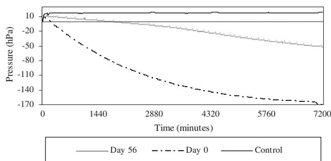
Fig. 4. Effect of incubation time on pressure drop on Day 0 and Day 56 of Treatment 2, Trial 1 (separated pig manure + sawdust) and blank control (no compost sample).
