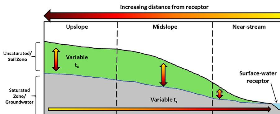
**Fig. 1.** Total time lag ( $t_T$ ) from source to receptor, including the unsaturated soil pathway ( $t_u$ ) and the saturated groundwater pathway ( $t_s$ ). Arrows indicate the variable duration of  $t_u$  and  $t_s$ , depending on the depth of the soil profile and proximity to a receptor, respectively.
