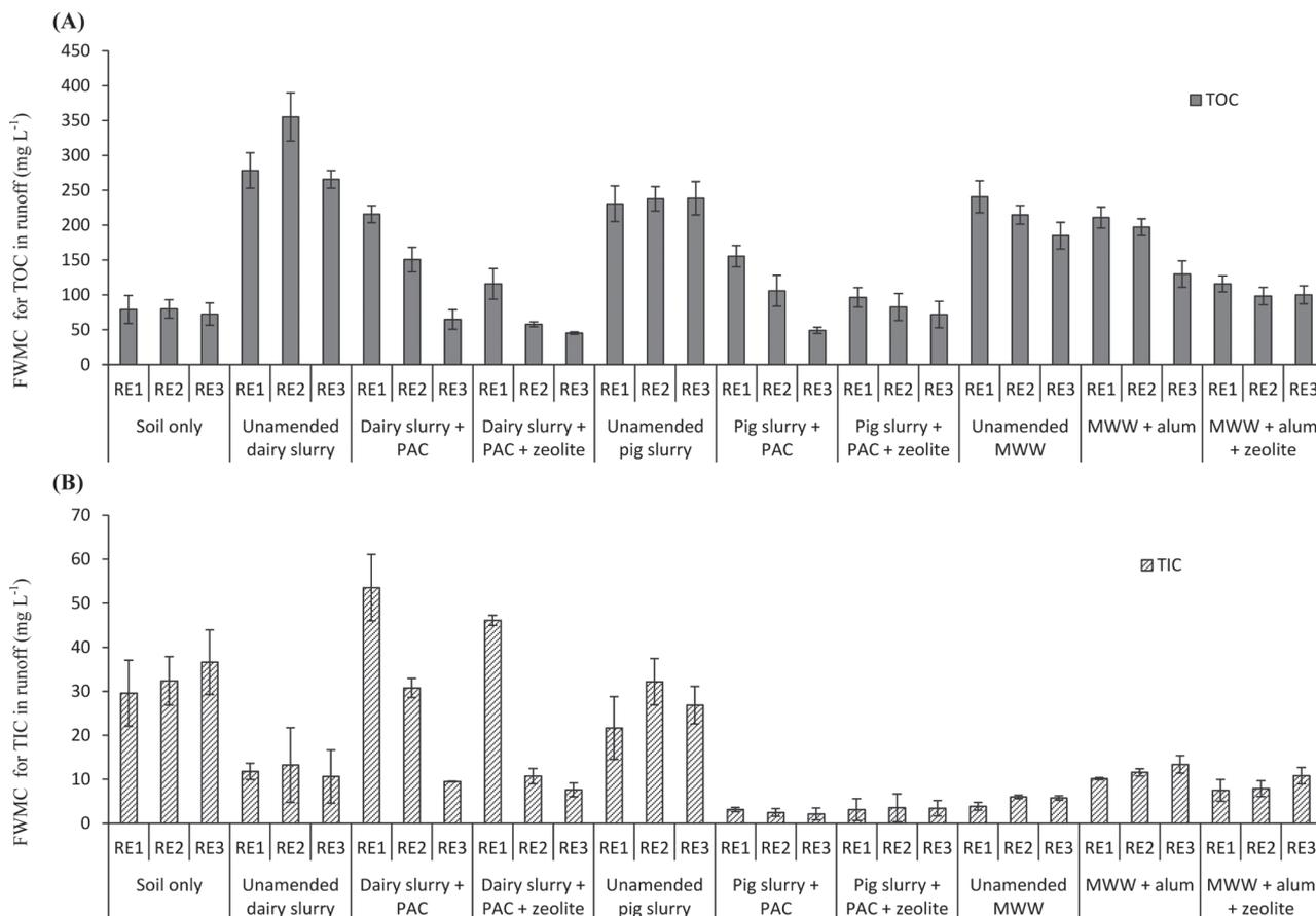
Fig. 2. Histogram of flow-weighted mean concentrations (FWMCs) ( $n = 3$ ) for (A) total organic C (TOC) and (B) total inorganic C (TIC) in runoff from rainfall event 1 (RE1) at  $t = 72$  h, rainfall event 2 (RE2) at  $t = 92$  h, and rainfall event 3 (RE3) at  $t = 120$  h. Error bars indicate SD.
