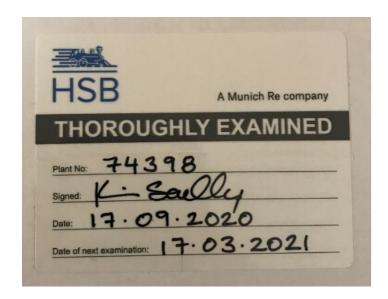
These tags will be fixed to the item and will display the Plant Serial Number, the signature of the person that has completed the examination, the date the examination was completed and the date of the next examination.
