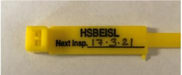
Fixed Sticker type Tag: Fixed Pressure and Lifting Equipment – for example Passenger/Goods Lifts, Fork Lift Trucks, Hot Water Boilers, Autoclaves etc.,
