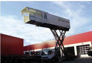
Positioning of catering trucks at Airbus A380
