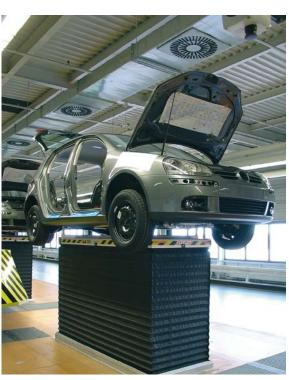
Height of lifting platforms on automobile production lines
