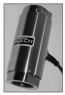
The F317 is a high performance cylindrical loadcell offering a high degree of output symmetry in compression and tension. A high slenderness ratio strain section improves all round performance compared to the older design F204. New thread sizes are employed offering more economic sizing of rod end bearings and improved availability. Novatech can supply suitable rod ends.
