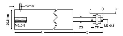
Our captive guided displacement transducer has bearings to guide the armature inside the measurement sensor. Captive LVDTs are for position measurement applications where guidance may be poor and end bearings may be required.
