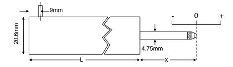
Our spring displacement transducer has bearings to guide the armature inside the measurement sensor and a spring which pushes the armature to the fully out position. Spring return LVDTs are appropriate where it is not possible to connect the transducer armature to the moving component being measured.
