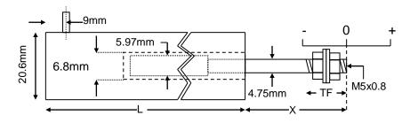
On our unguided LVDTs the armature assembly is a separate component, to make a measurement the user must guide the armature inside the body without touching the sides. Unguided position measurement transducers are appropriate where external guidance is available and give truly non-contact operation
