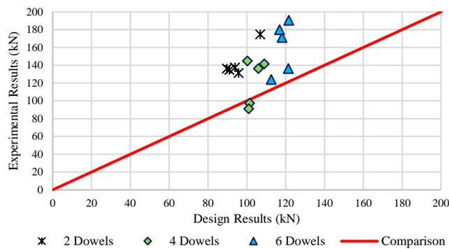
Figure 8.1 Comparison of design and experimental results.
