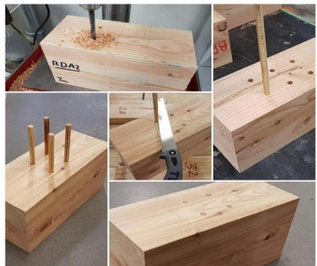
Figure 5.2 Specimen preparation
