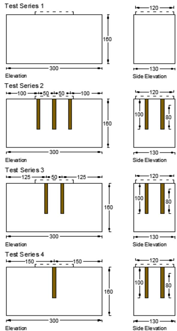
Figure 5.1 Specimen Layout
