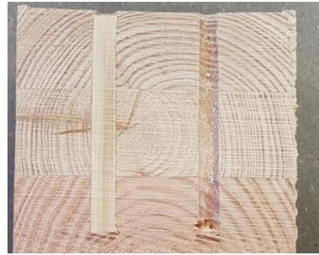
Figure 7.5 Specimen with failure of the adhesive bond
