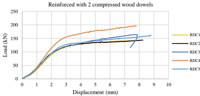
Figure 7.4 Load-deformation for specimens with 2 dowels
