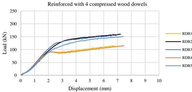
Figure 7.3 Load-deformation for specimens with 4 dowels
