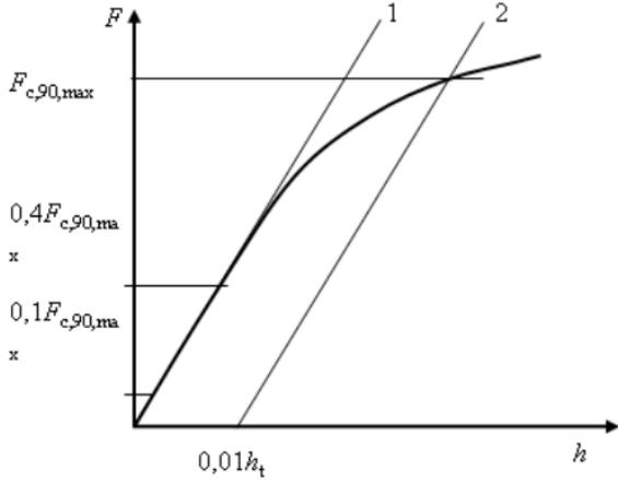
Figure 2.1 Load-deformation curve [7]
