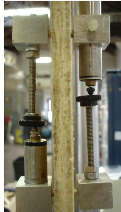
Fig. 2(b) – Full-bridge LVDT's mounted to the test piece using custom made mounting blocks
