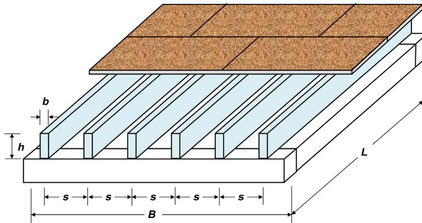
Fig. 9. A typical floor constructed with solid timber joists.
