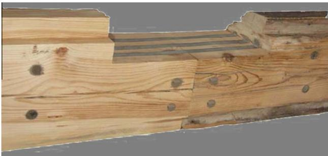
Fig. 6. Shear reinforcement with GFRP.
