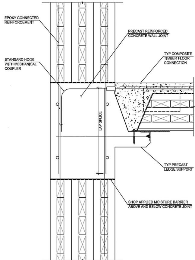
Figure 15. SOM concrete joint detail (SOM, 2013).
