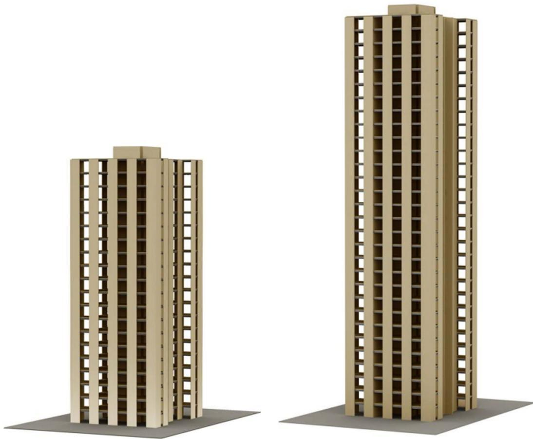
Figure 13. FFTT building frames: Options 3 (20-storey) & 4 (30-storey) (Green, 2012).
