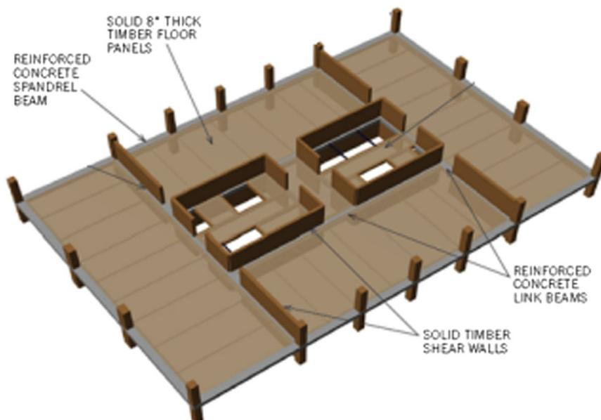
Figure 14. SOM concrete-jointed timber frame (SOM, 2013).
