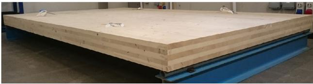
Figure 1. 5-layer CLT floor panel.
