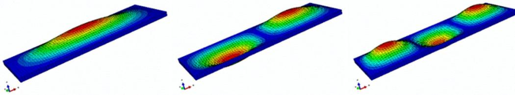
Figure 19. Mode-shapes of two-way spanning CLT panels (Uí Chúláin et al., 2016).
