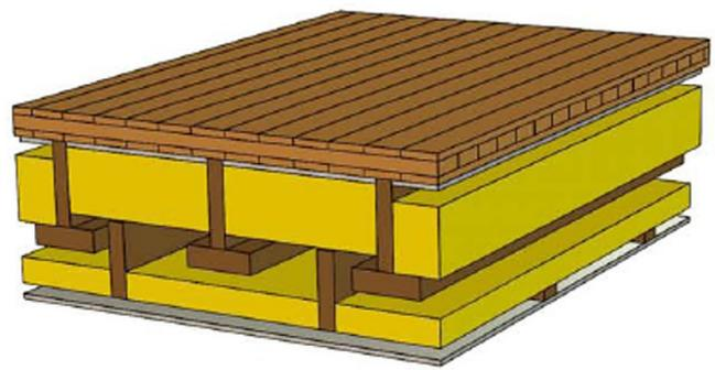
Figure 8. Limnologen floor-ceiling detail (Serrano, 2009).
