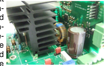
Micro-Processor controlling 144 battery cells using the newly developed SEICC regime
