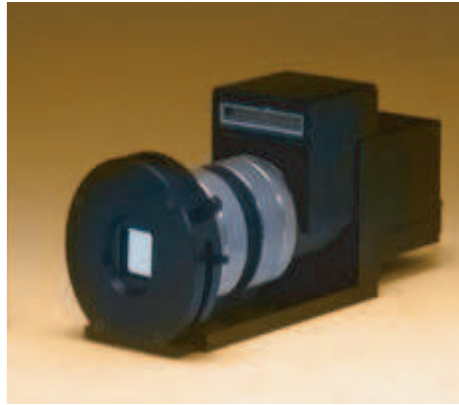
Fig. 6.6: Hamamatsu SLM used to generate Zernike aberrations.
