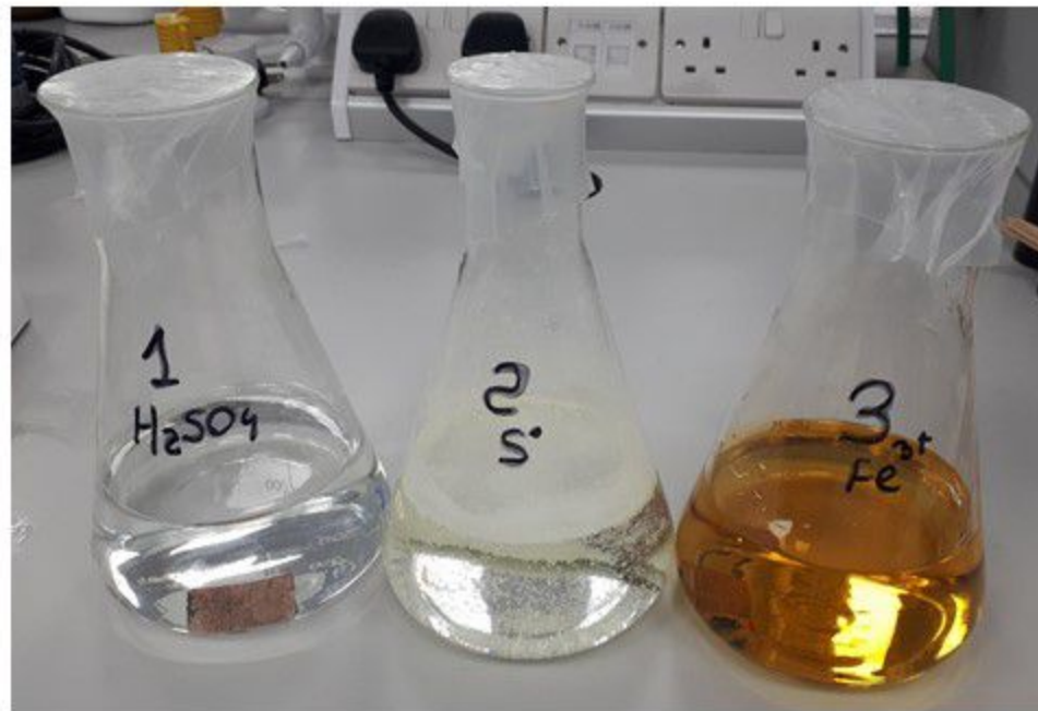
Leaching media and PCB before leaching process
