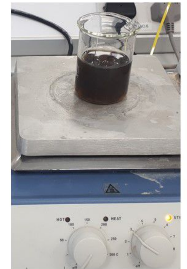
Leaching solution during metal precipitation
