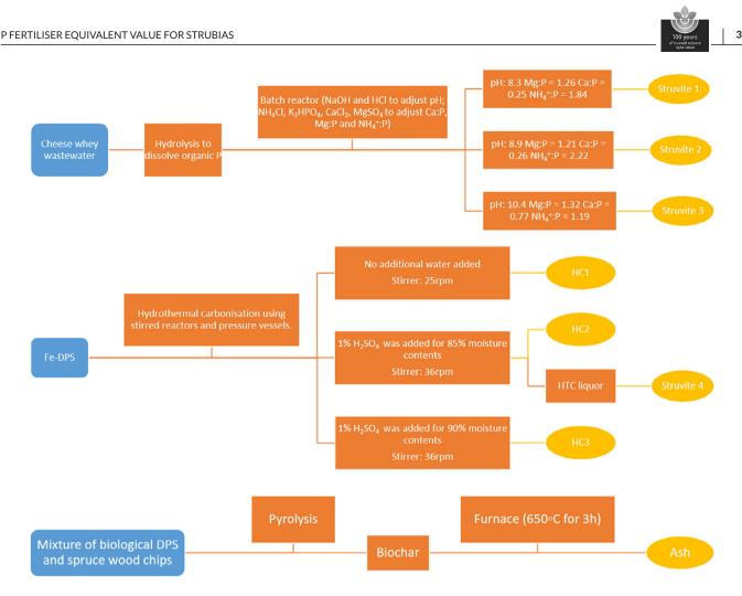
**FIGURE 1** Production stream of struvite, biochar and ash (STRUBIAS) fertilisers production. Abbreviations used in diagram: DPS, dairy processing sludge; HC, hydrochar; HTC, hydrothermal carbonisation.
