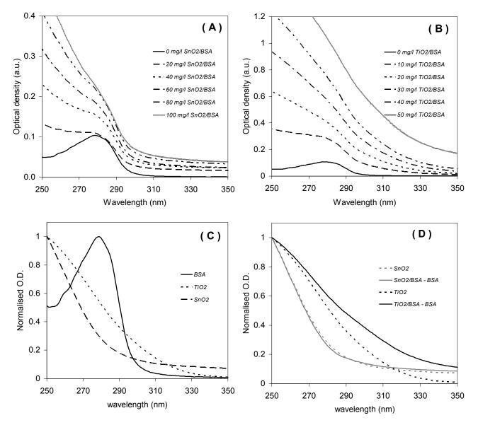
Fig. 2. UV absorption spectra of BSA with SnO<sub>2</sub> (A), and TiO<sub>2</sub> (B) nanoparticles at different concentrations. The Nanoparticle normalised UV spectra at 250 nm is displayed with normalised BSA UV spectrum in (C). The normalised mathematical subtracted spectra for BSA/SnO<sub>2</sub> and BSA/TiO<sub>2</sub> mixture by BSA spectrum is displayed with normalised 50 mg/l TiO<sub>2</sub> and 100 mg/l SnO<sub>2</sub> NP's (D).
