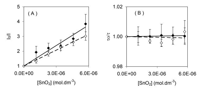
Fig.6. Stern-Volmer plots Io/I (Panel A) and  $\tau_0/\tau$  (Panel B) against SnO<sub>2</sub> nanoparticle concentration. The solid symbols represent the quenching data of BSA, while NAT quenching data are represented by open symbols. The solid lines are the best curve fit for BSA fluorescence quenching using eq.4 and the dashed line for NAT fluorescence quenching using eq.4.
