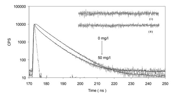
Fig.4. Time resolved fluorescence decay of 2.5  $\mu$ M BSA at different concentrations of TiO<sub>2</sub> nanoparticle. (Grey lines), biexponential fit (dark lines), and the instrument response function (dotted line). The inset figure shows the residues from the fit. Data collected at 295 nm excitation with the emission measured at 340 nm and a channel resolution of 70 ps.
