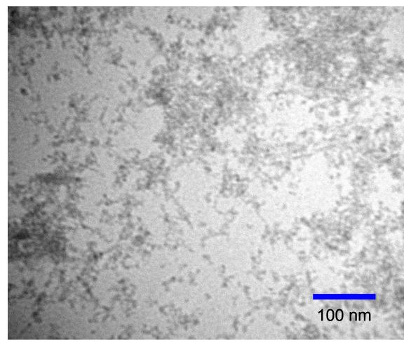
Fig. 1. Transmission Electron Microscopy images of SnO<sub>2</sub> nanoparticles magnified 200k times.
