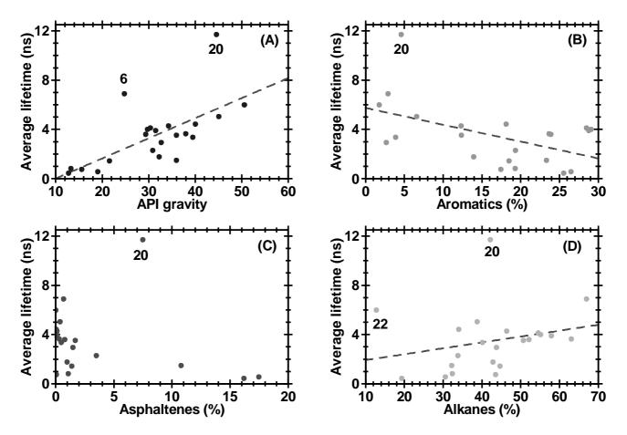
Figure 2: Plots of average fluorescence lifetime versus: (A) API gravity; (B) Aromatic concentration (% by weight); (C) Asphaltene concentration (% by weight); (D) Alkane concentration (% by weight). All data acquired at an emission wavelength of 450 nm using 380 nm excitation.
