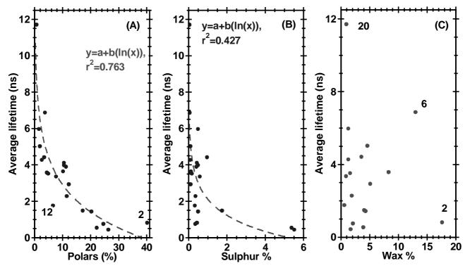
**Figure 3:** Plots of average fluorescence lifetime versus: (A) Polar concentration (% by weight); (B) Sulphur concentration (% by weight); (C) Wax concentration (% by weight); All data acquired at an emission wavelength of 450 nm with 380 nm excitation.
