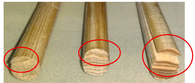
Fig. 2. Interlaminar shear failure of the CW dowels.
