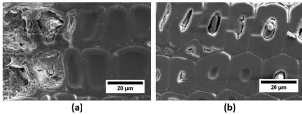
(a) normal and (b) compressed Scots Pine at a magnification of 5000X
