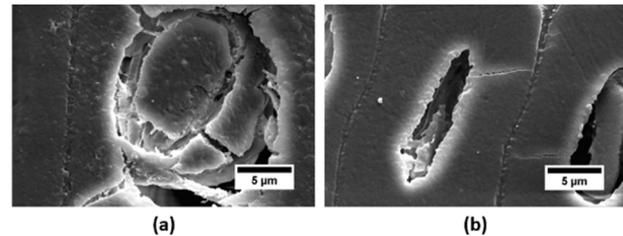
(a) normal and (b) compressed Scots Pine at a magnification of 15000X
