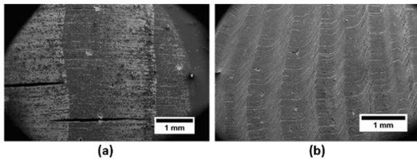
(a) normal and (b) compressed Scots Pine at a magnification of 75X
