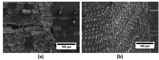
(a) normal and (b) compressed Scots Pine at a magnification of 1000X
