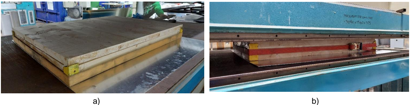
Figure 4: CLT panel manufacture, a) panel adhesive application and lay-up, b) the CLT panel is subjected to a specific pressure while the adhesive cures
