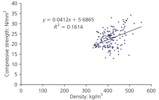
Figure 3. In-grade compressive strength plotted against density
