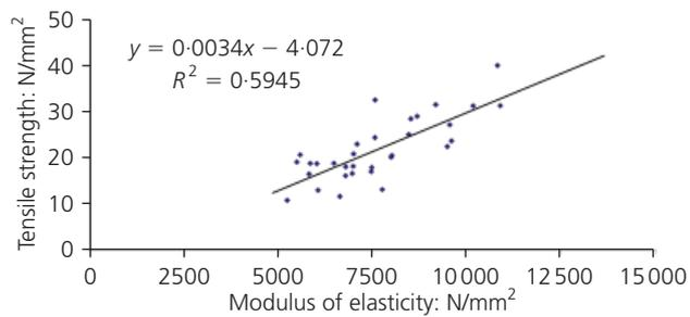
Figure 7. In-grade tensile strength plotted against modulus of elasticity
