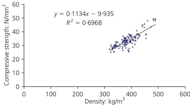
Figure 1. Clear wood compressive strength plotted against density
