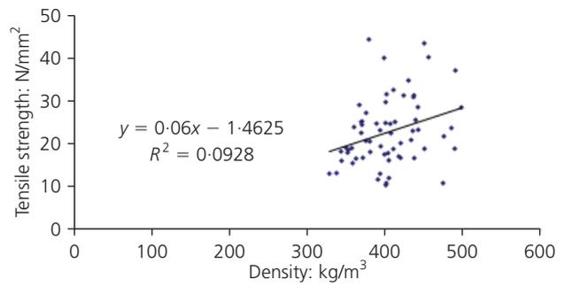
Figure 9. In-grade tensile strength plotted against density
