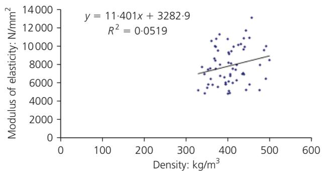
Figure 11. In-grade modulus of elasticity plotted against density
