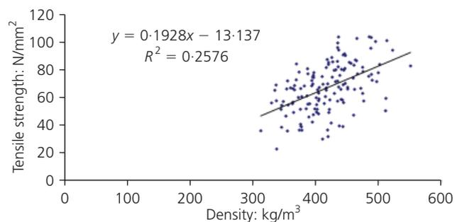
Figure 4. Clear wood tensile strength plotted against density
